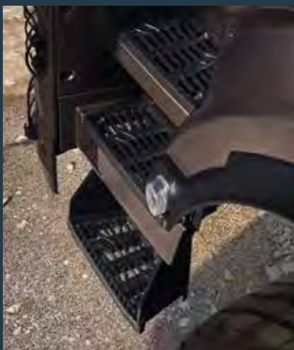
Lowest step fitted with a swing-type function made out of an especially elastic plastic
