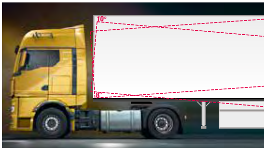
Angle of inclination of fifth-wheel coupling at 150 mm height and tyres 315/70 R 22.5
