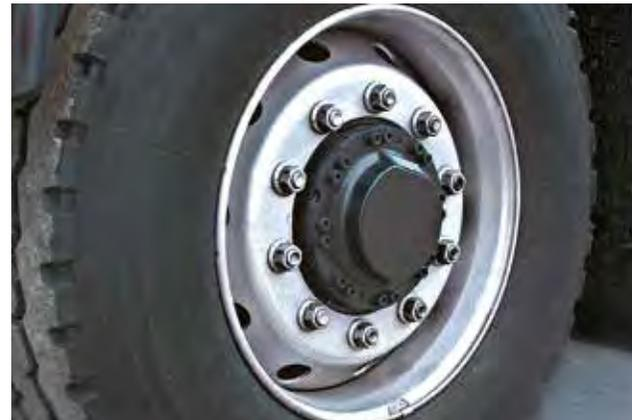
Front axle with hydrostatic wheel hub motors
